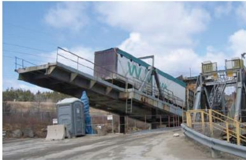
Figure 10.3 Biomass carrying truck is tilted to unload biomass in the plant. (Photograph by the author)
